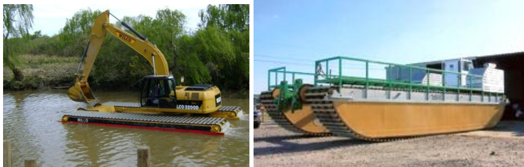
Figure 3. Amphibious equipment: A marsh buggy (left) and a cargo buggy (right)
